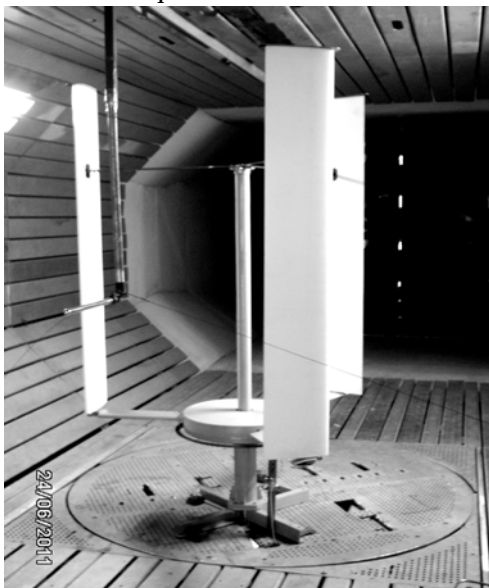
Fig.1. The wind turbine with controlled blades in the wind tunnel
